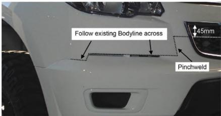
It is suggested you remove the front grille off the car inorder to make the final cut shown below. You will need to remove the 2 barbs either side under the head lights with bolt cutters or grinder, do not grind near colour coded bullbar
