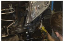
8. Carefully mount the Extreme Series bar it is best to get someone to help you. The bulbar alignment can be difficult. Its best to have bolts loose enough so two persons can hold the bar in place while a 3<sup>rd</sup> tightens the bar. If you are installing by your self alignment can be difficult its suggested you tighten 1 side enough so it can still move under pressure and wedge foam (or similar) between bar and fender to retain gap when lifting the other side into place.
